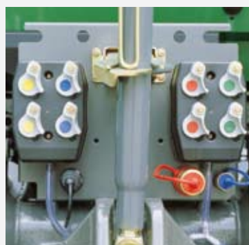
Double-sided connect-under-pressure couplings; external load-sensing hydraulic connection
