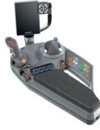
The multifunction armrest with Power equipment and Varioterminal 7-B; Power joystick with VarionicTI headland management, cruise control keys and engine speed; EPC operating module for rear power lift, PTO; The Varioterminal 7-B in smartphone look with real glass surface offers an excellent overview of all functions, an intuitive menu navigation, touch and key control as well a ISOBUS implement control.
