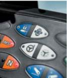
All functions are arranged simply and clearly on the backlit membrane keypad according to the tried and tested Fendt
