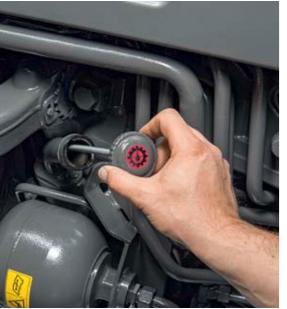
Maintenance activities, such as checking the oil level or changing the filter, are performed quickly and easily on the Fendt 1000 Vario. The engine compartment is especially easy to access thanks to the removable side panels.
