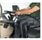
For enhanced operating comfort, the cockpit swings parallel with the steering wheel.
