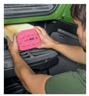
The cab filter is well accessible in the entry area and can be easily cleaned, when necessary.
