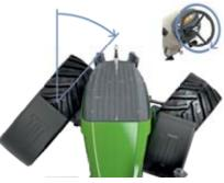
Hand brake assistant in automatic position: The hand brake is automatically activated.
