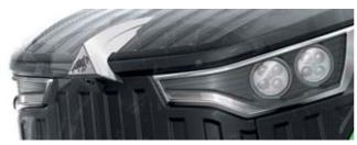
LED daytime running lamps and work lights integrated in the front of the bonnet including bonnet camera.
