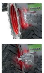
The Fendt 1000 Vario offers a flanged axle or an axle stub variant to meet different requirements.
