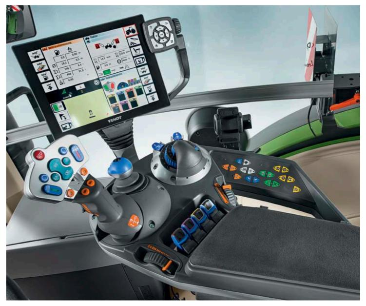
The operating elements on the right-hand armrest – the 4-in-1 Varioterminal, multi-function joystick, crossgate lever, EPC power lift module, valve operation and membrane keypad – have a well-balanced overall design and form an ergonomic command centre where everything is under control.
