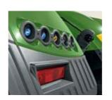
The external valve actuation allows you to control the rear power lift, one valve and the PTO directly on the rear mudguard.
