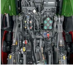
The Fendt 1000 Vario can be customised by upgrading or downgrading. The fully equipped rear has all the connections and functions, such as power beyond, ISOBUS socket, rear return, PTO and rear linkage.
