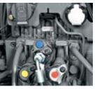
The DCUP couplings permit all hydraulic valves to be coupled under pressure on both sides. The pressure relief lever permits easy coupling.
