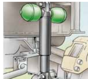
Rear hydro-pneumatic self-levelling suspension
