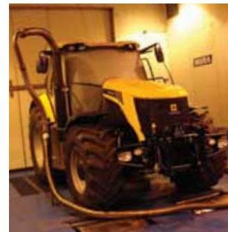
Hot cell testing
