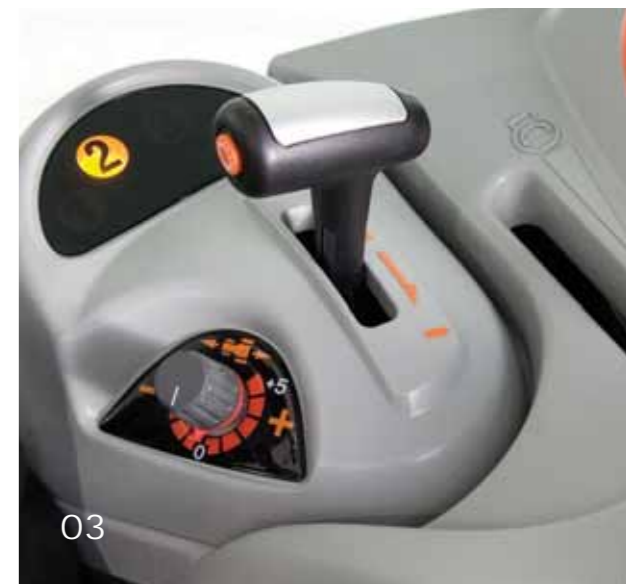
01 The Dyna-4 transmission offers four Dynashift changes in each range, excellent ground speed 'overlap' and 40 km/h maximum speed for efficient haulage operations. (40 km/h can be reached with 38, 34 or 30 inches tyres).
