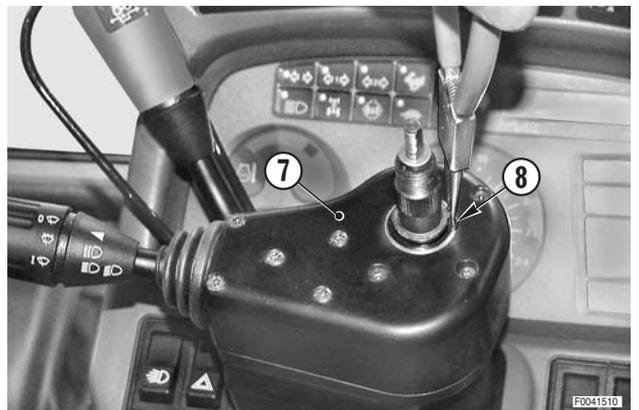
5 - Lift off the switch unit (7) and place it to one side.
