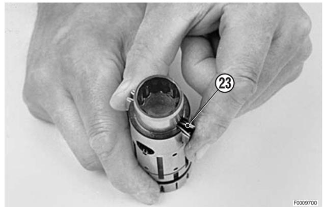
3 - Insert the inner sleeve (17a) in outer sleeve (17b).
