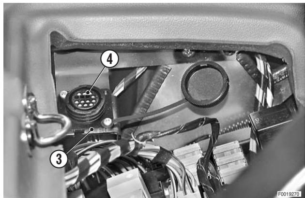
4 - Disconnect the connectors (P2), (P6), (P3), (P5), (J1), (J2) and (J3) from the fuse/relay board.
