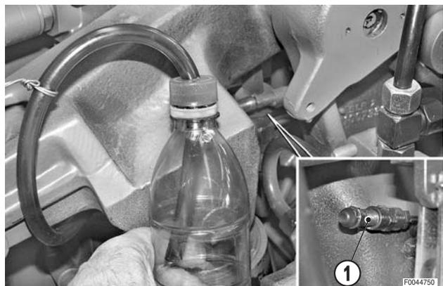
9 - Bleed the braking valve at the bleed screws (1) (protected by caps) using the method indicated for the pumps and choosing from among the following versions:
