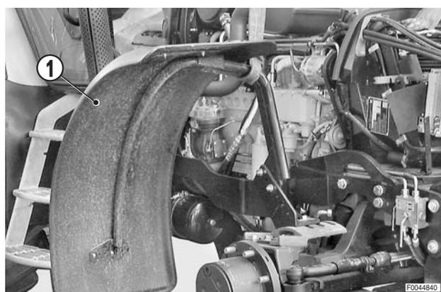
3 - Unscrew and remove the bolts (2) and remove the fender (1) complete with the mounting bracket (3).
