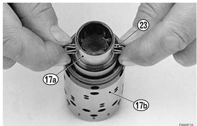
5 - Align the springs (23) and position them centrally relative to the diameter of the outer sleeve (17b).
