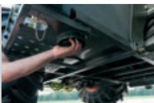
Large opening for cleaning
